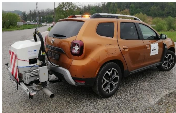
Figure 3. Test vehicle with built-in measuring equipment
