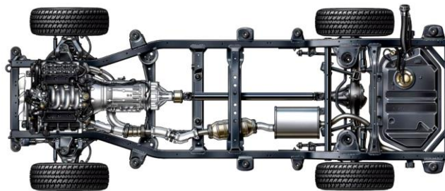
Figure 2: Chassis and drivetrain layout of traditional rear-wheel drive vehicle (Vallance, 2011).
