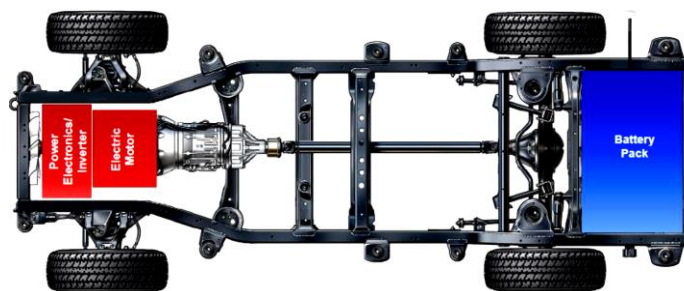
Figure 3: Chassis and drivetrain layout of a retrofitted electric vehicle with OWM (Vallance, 2011).
